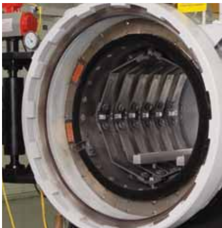
TITAN'S STANDARD ALL-GRAPHITE HOT ZONE WITH CFC HOT FACE
