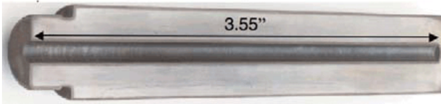
Figure 3: Example of Blind Hole
