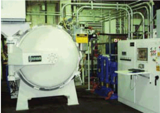
Figure 7: Two Chamber Design: Oil and/or Gas
